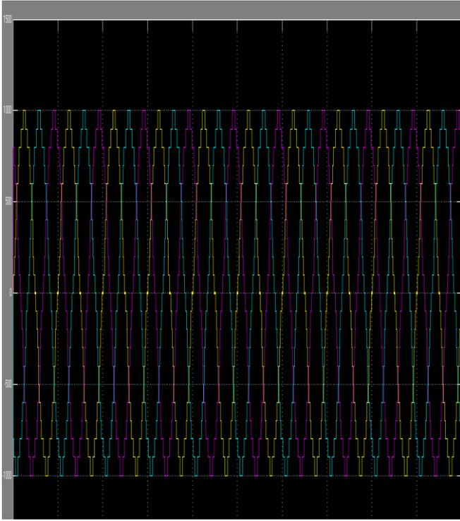
Fig.7. 21-Level voltage waveform
