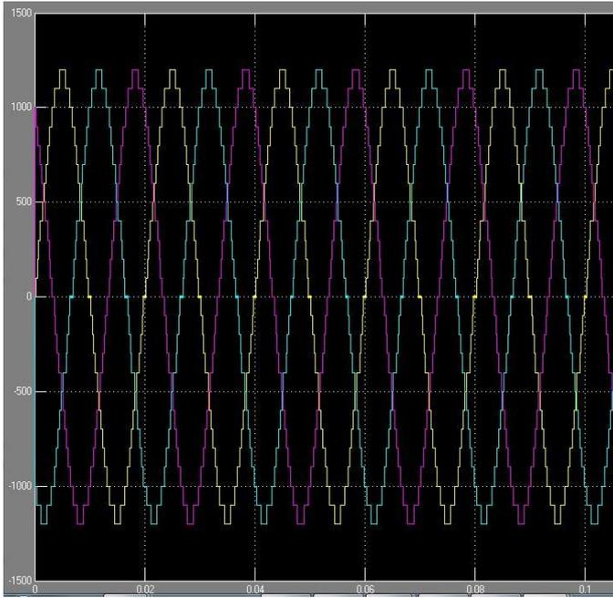
Fig.15. 25-Level Voltage waveform
