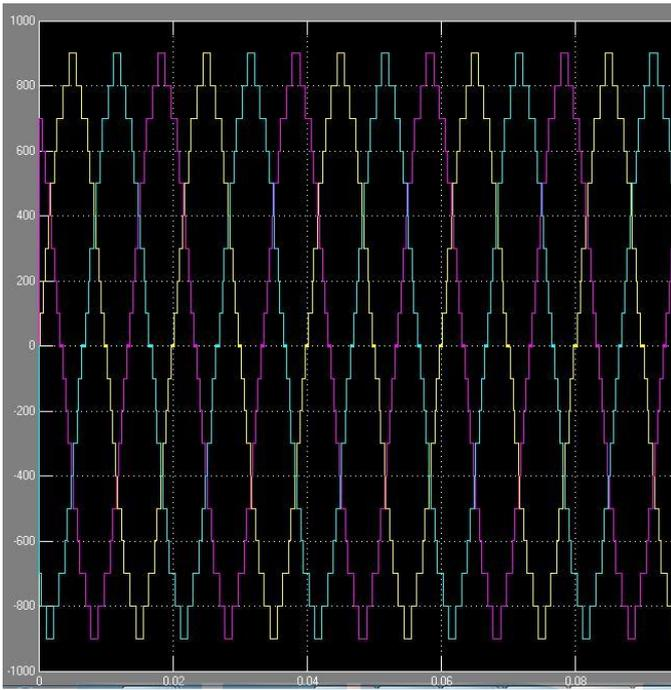
Fig.11. 19-Level voltage waveform
