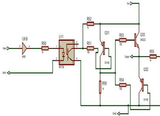
Fig.5 Driver Circuit
