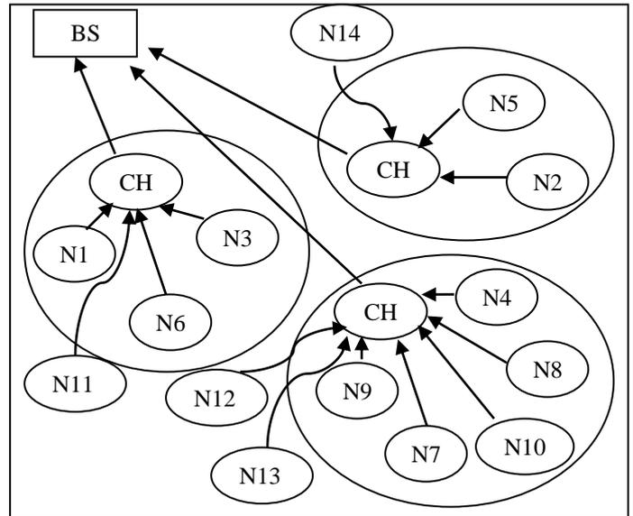
Fig2: LEACH-MAE Protocol Architecture
