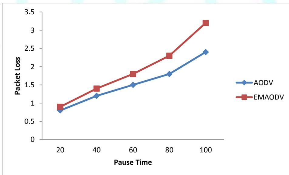
Figure 2: packet loss vs. pause time of AODV & EMAODV
