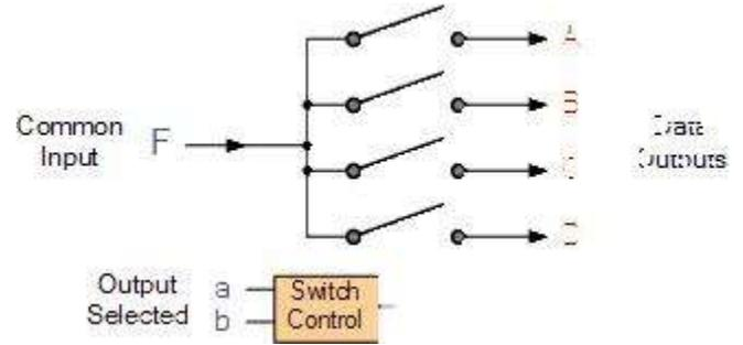
Demultiplexers take one data input and a number of selection inputs, and they have several outputs. They forward the data input to one of the outputs depending on the values of the selection inputs. Demultiplexers are sometimes convenient for designing general
