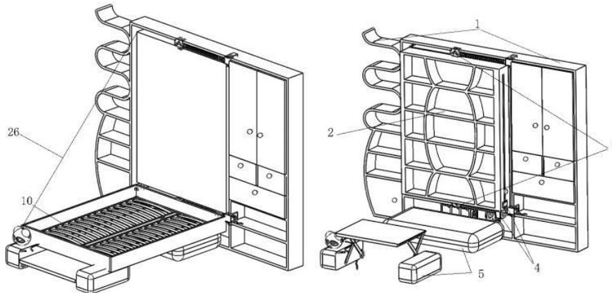
Fig. 5 Schematic diagram of lifting mechanism
