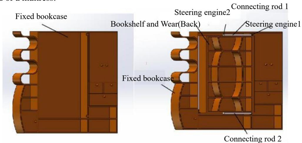
Fig. 2 Support diagram of the main body of the fixed bookcase
