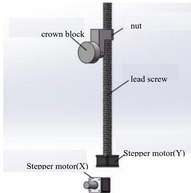
Fig. 6 Traction device (internal)
