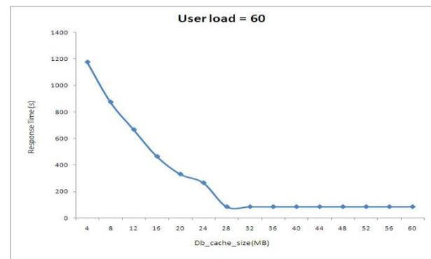
Figure 2. Effect of Buffer cache on Response time(DSS)
