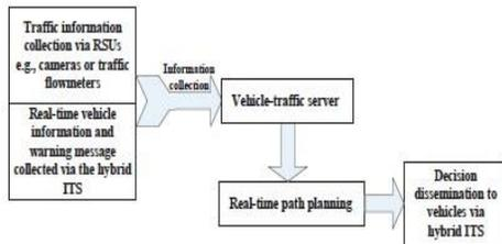
Figure 3: Path planning in a VNET-enhanced ITS
