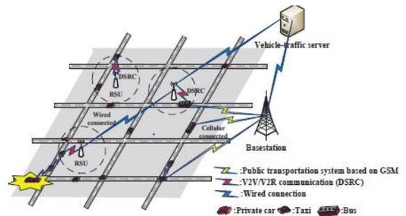
Figure 2: Hybrid VANET-enhanced network architecture
