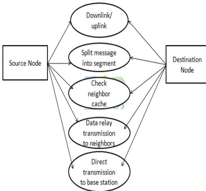
Fig.1: Data Transmission in the DTR protocol
