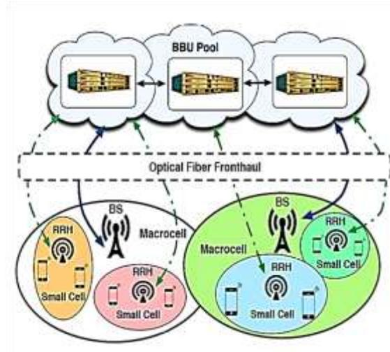
Figure 6: Cloud Radio Access Network Architecture
