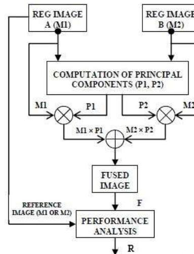
Fig 2: Flowchart of PCA Algorithm
