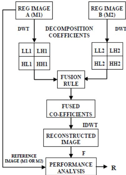
Fig 1: Flowchart of DWT Algorithm
