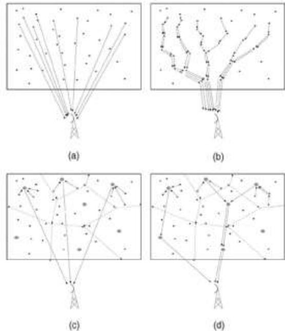
**Figure: 4** Sensor information forwarding with and without clustering and aggregation. (a) Single hop without clustering. (b) Multihop without clustering. (c) Single hop with clustering. (d) Multihop with clustering.
