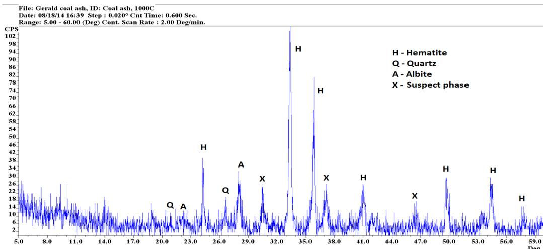
Coal powder was fired at 1000°C for 2 hours; the resulted ash was analyzed by XRD. Major mineral: hematite
