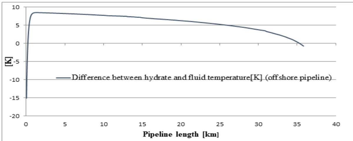
Figure 4. Difference between hydrate and fluid temperature in the offshore pipeline.
