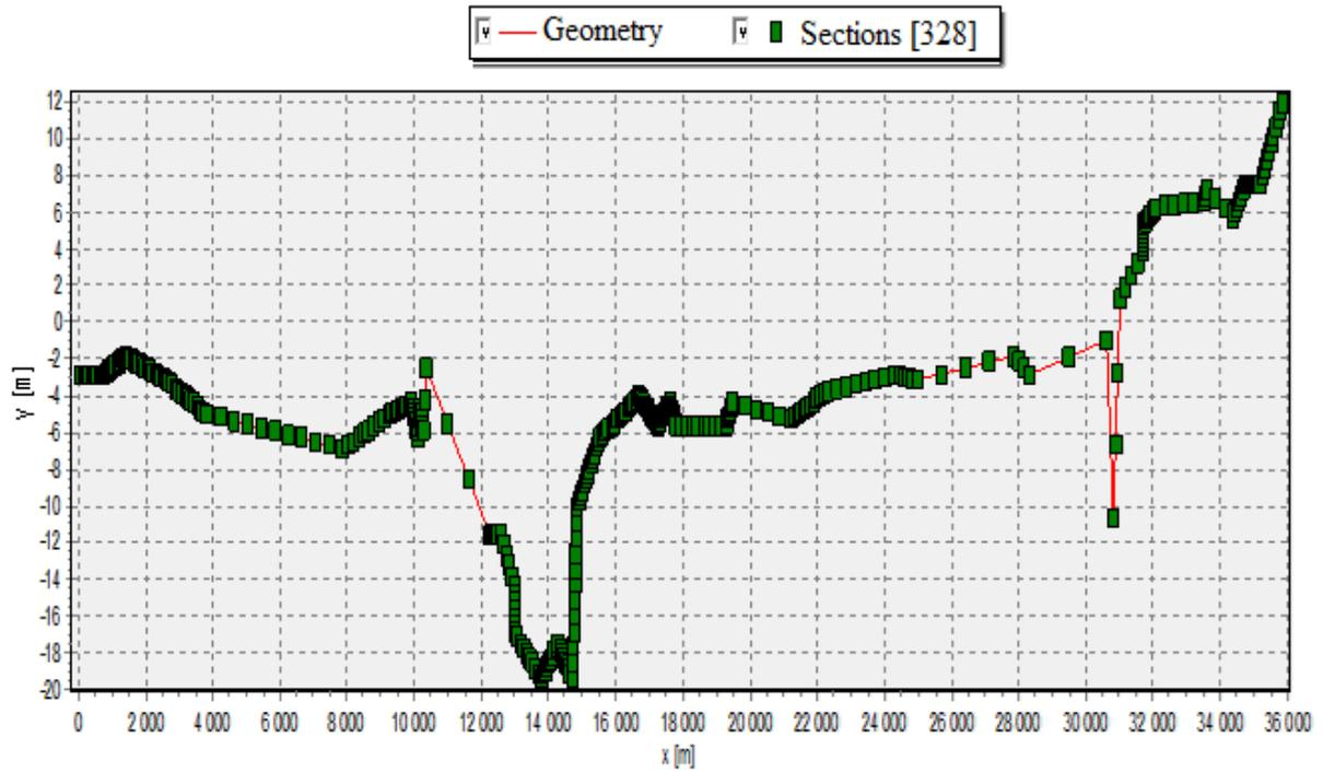
Figure 2. Geometry of the offshore pipeline generated by OLGA software.
