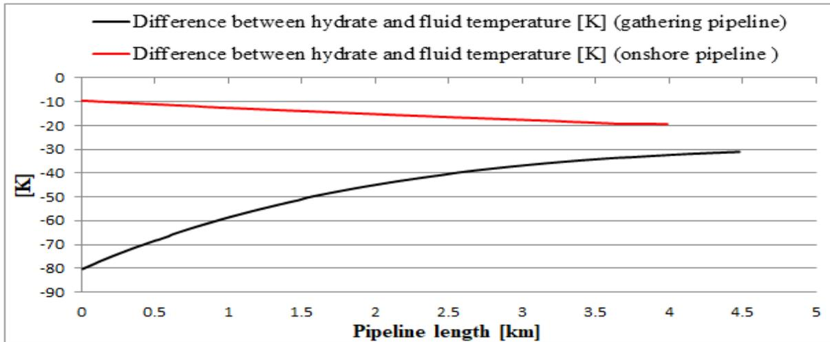
Figure 5. Difference between hydrate and fluid temperature in the onshore and gathering pipeline.
