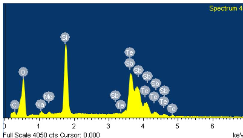
Figure 8. EDS spectrum of RF2 sample that shows the elements of  $\text{Sb}_2\text{Te}_3$  and glass.
