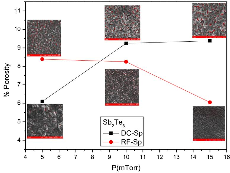
Figure 9. % Porosity of the  $Sb_2Te_3$  thin film vs. deposition pressure for DC and RF-Sp.
