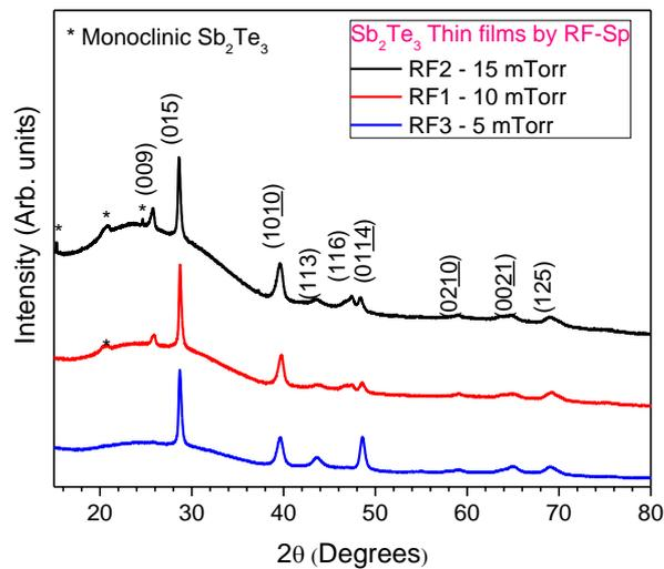
Figure 3. XRD patterns of  $Sb_2Te_3$  thin films deposited by RF-Sp at different pressure.
