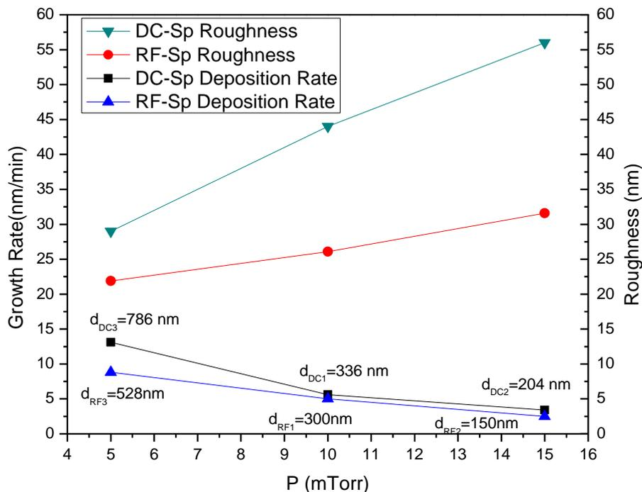
Figure 1. Thickness, roughness and growth rate for  $Sb_2Te_3$  thin films deposited by DC and RF Sputtering system as a function of deposition pressure.
