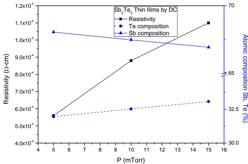
Figure 6. Resistivity and Sb, Te atomic composition for  $Sb_2Te_3$  thin films deposited by DC-Sp as a function of deposition pressure.
