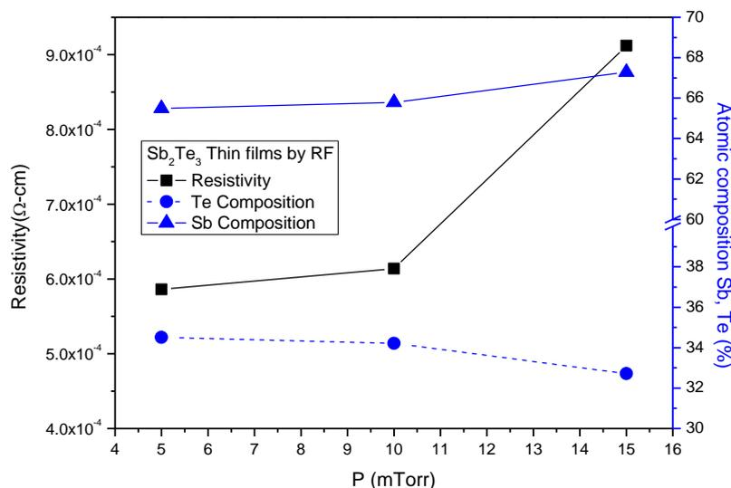
Figure 7. Resistivity and Sb, Te atomic composition for  $Sb_2Te_3$  by RF-Sp as a function of deposition pressure.
