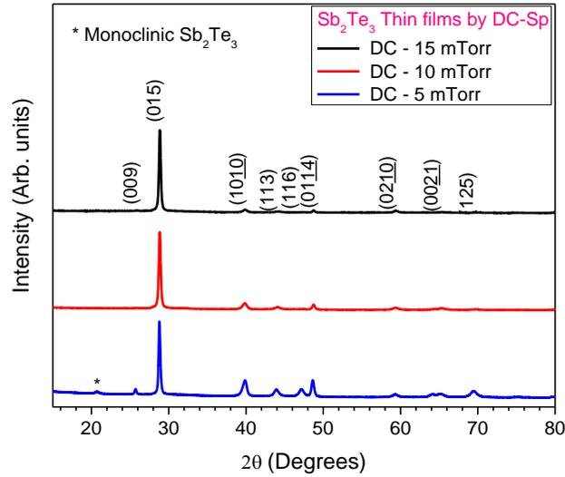
Figure 2. XRD patterns of  $Sb_2Te_3$  thin films deposited by DC-Sp at different pressure.
