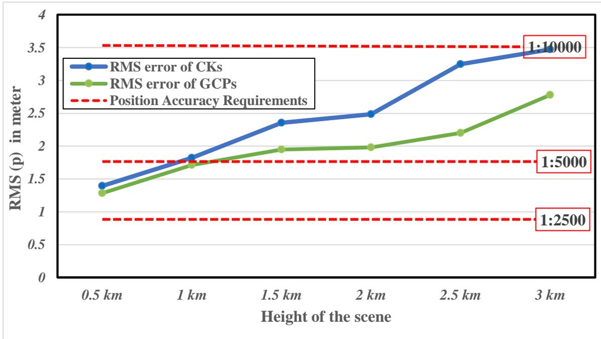
**Figure (3): The relationship between RMS error at different height of the scene and position accuracy requirements for different maps**
