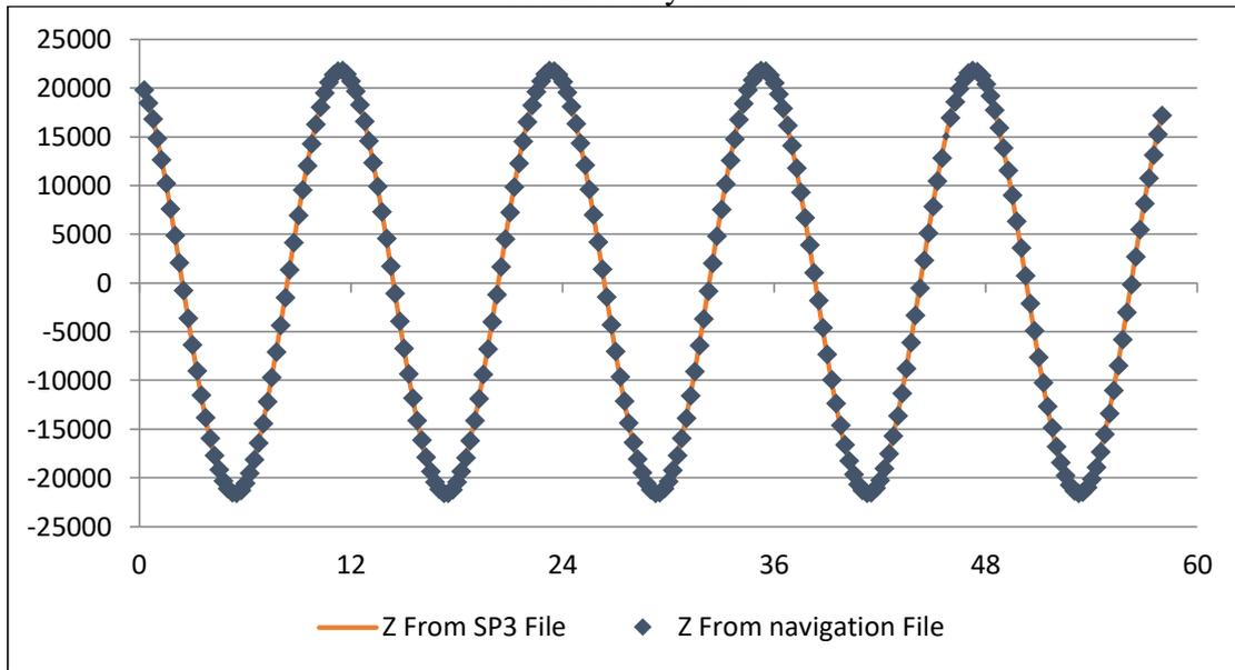
Figure 4. Relationship between time in hours as x axis and  $Z_{ECEF}$  coordinates in km for satellite as y axis
