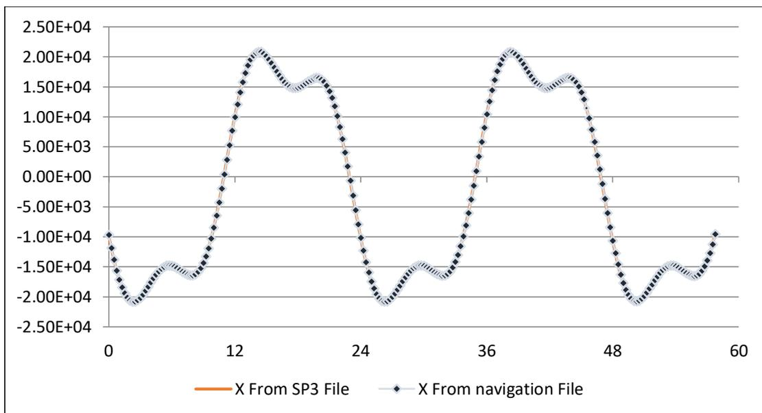
Figure 2. Relationship between time in hours as x axis and  $X_{ECEF}$  coordinates in km for satellite as y axis
