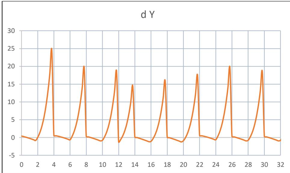
Figure 6. The difference between the precise and broadcast orbits in  $Y_{ECEF}$  direction
