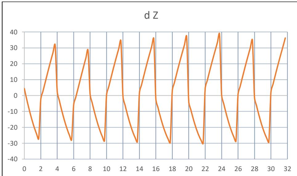
Figure 7. The difference between the precise and broadcast orbits in  $Z_{ECEF}$  direction
