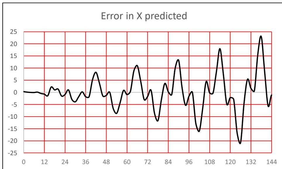
Figure 8. Errors in calculating orbit. Horizontal axis is time in hours and errors in predicted  $X_{ECEF}$  in ms is y axis
