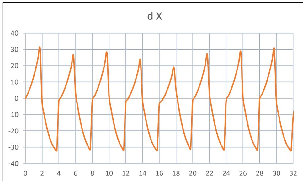
Figure 5. The difference between the precise and broadcast orbits in  $X_{ECEF}$  direction
