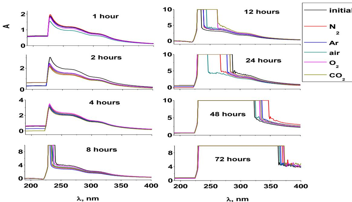
Fig. 8. UV spectra of the medium swelling on successive stages of artificial aging of seeds wheat in water with gas nanoparticle.
