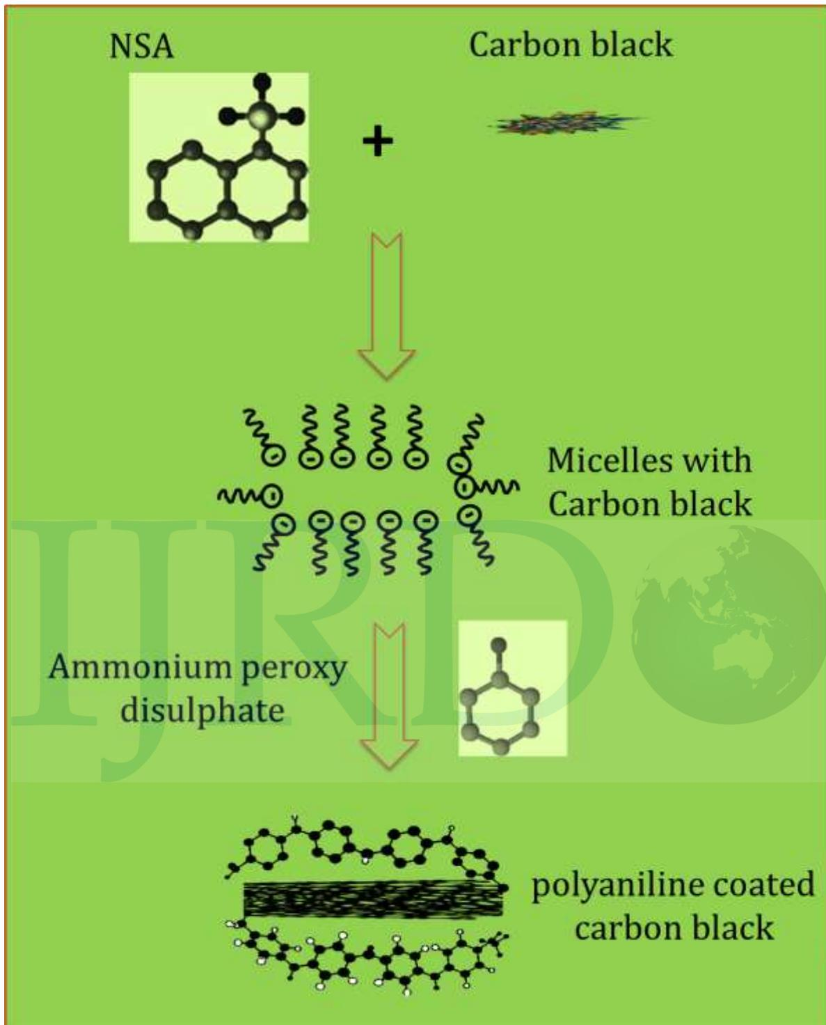
**Figure 2.** Schematic representation of the PANI/carbon black composite
