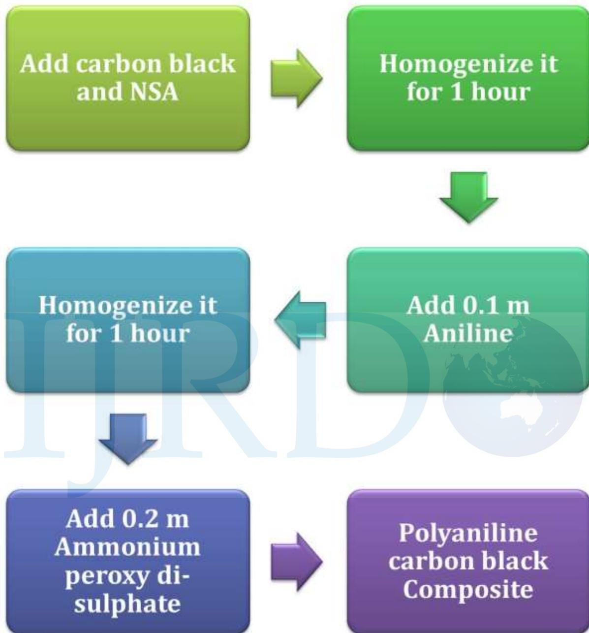
**Figure 1.**Flow chsart of the synthesis procedure of PANI composite
