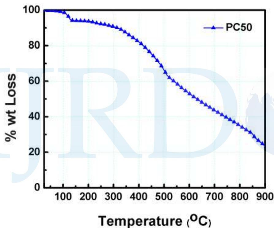
**Figure 5** Thermal gravimetric analysis of carbon black and PANI composite
