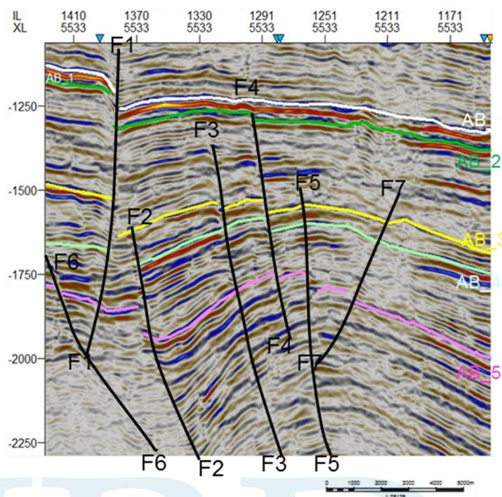
Fig. 4: Interpreted seismic section showing the mapped horizons and faults
