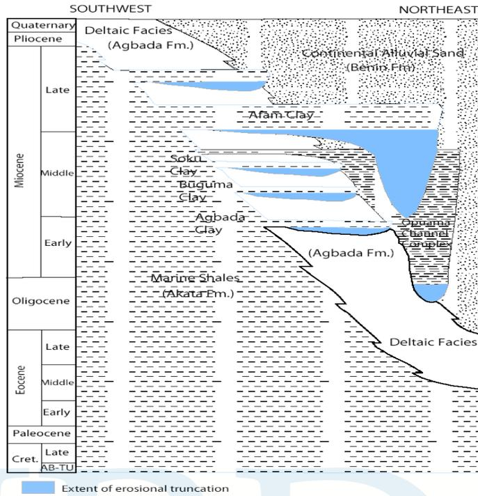
Fig. 2: Stratigraphic Column Showing the Three Formations of the Niger Delta. [After 7, 8]
